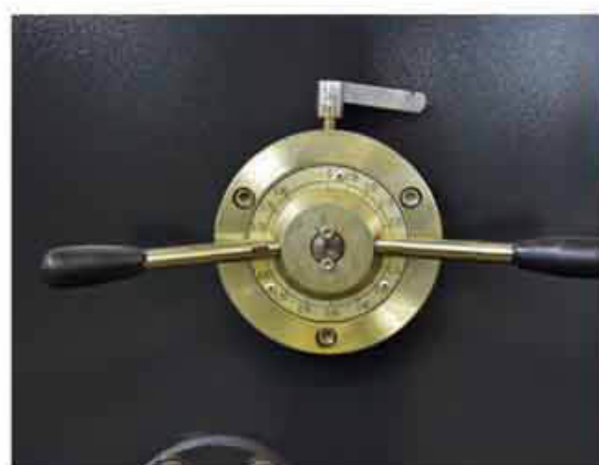
Manual quick change blade gap adjustment
