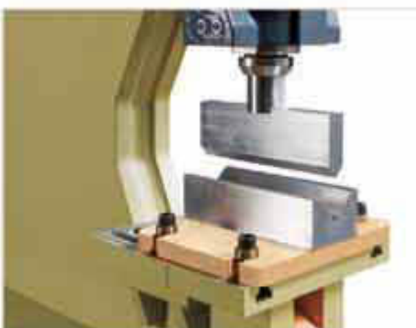
Lengthwise Installation of Bending Die
